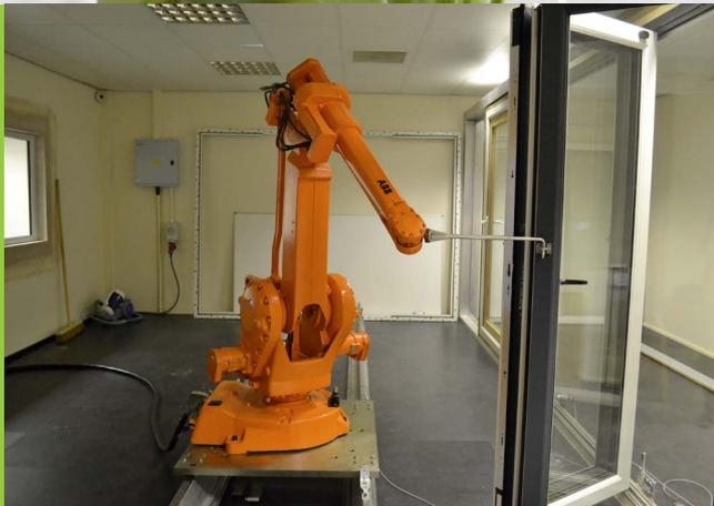
“ We've invested in a robot to mechanically open and close the doors, really putting the Liniar bi-fold through its paces – we want to prove they're definitely built to last ”
